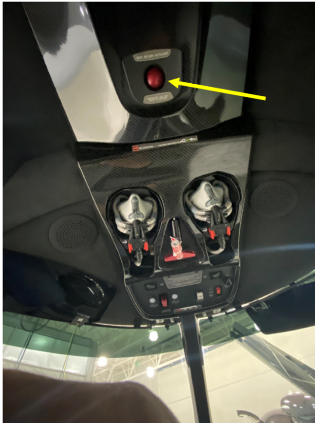
Figure 2 . – Yellow arrow shows location of Autoland pushbutton (Source: Cirrus Aircraft).
