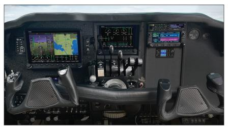
The Baron Dynon panel here has a 10-inch PFD and 7-inch MFD that also serves as an engine and fuel display. That's a PS Engineering PMA450B audio panel, Avidyne IFD440 (Garmin navigators work, too) and Dynon comm radio control head in the main stack. That's the Dynon auttopilot controller picture at the top of the page.
