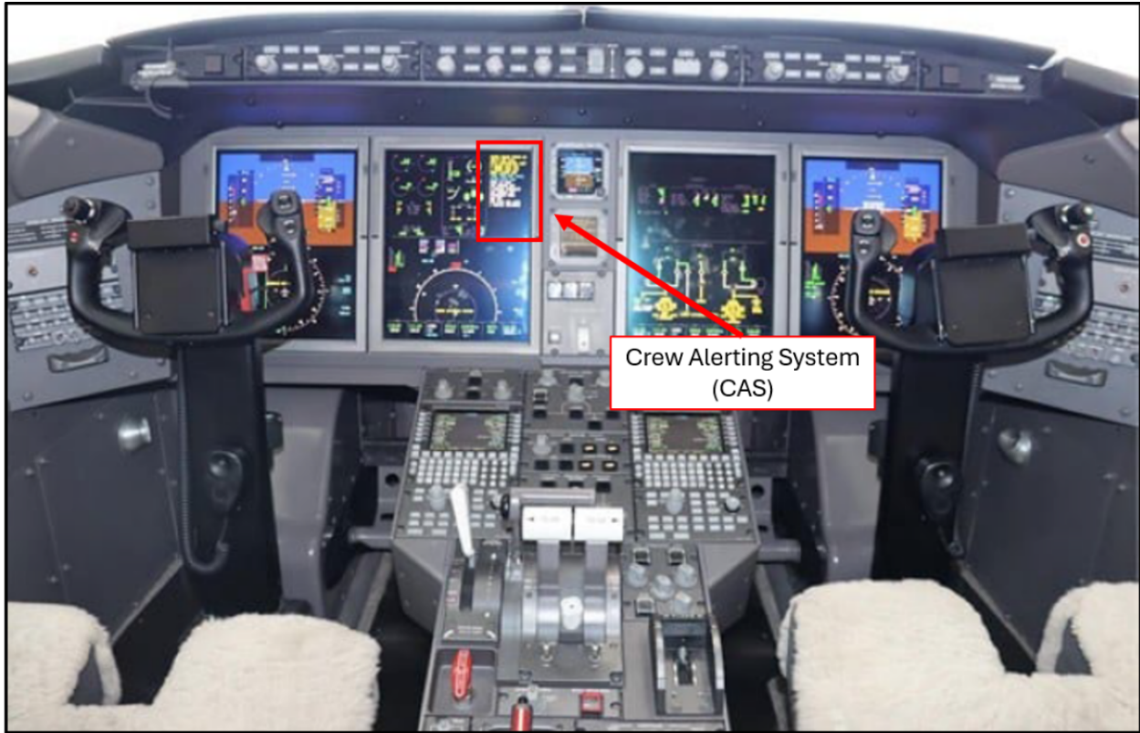
Figure 3: View of the cockpit in the accident airplane with the CAS location annotated (Source of Photo: Aircraft.com)
