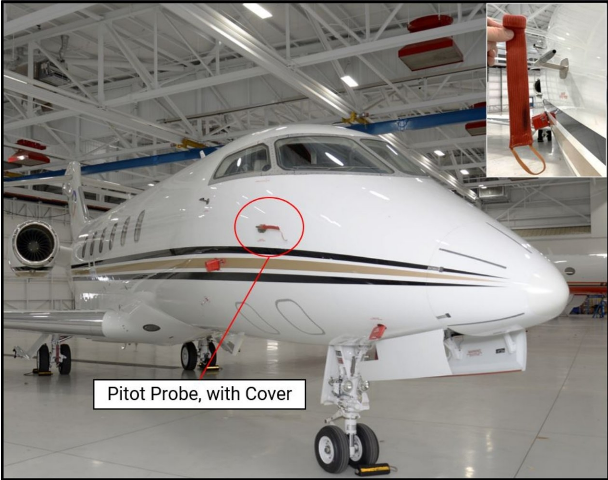
Figure 4: View of the right side forward area of the airplane showing the covered pitot probe.
