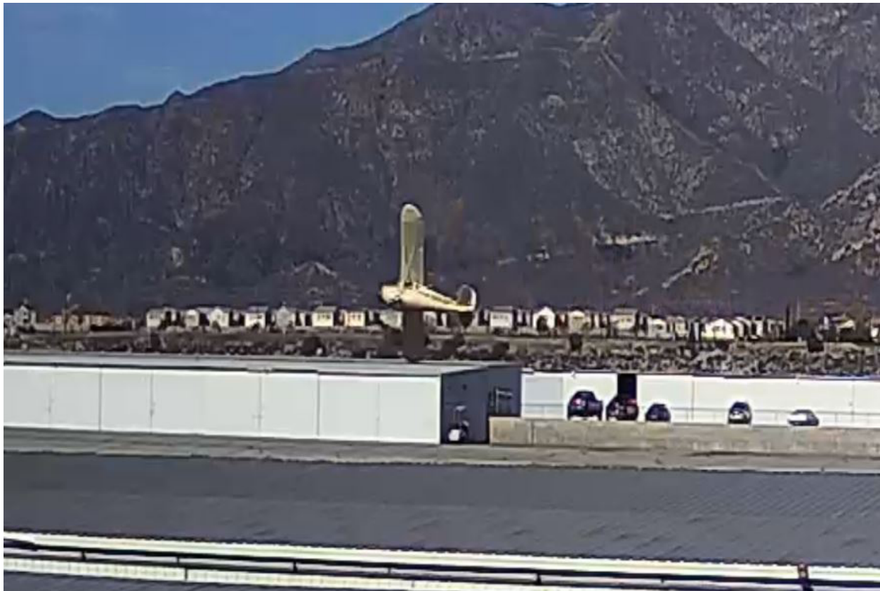
Opposite aileron can be seen here in an attempt to stop the aircraft from rolling.
