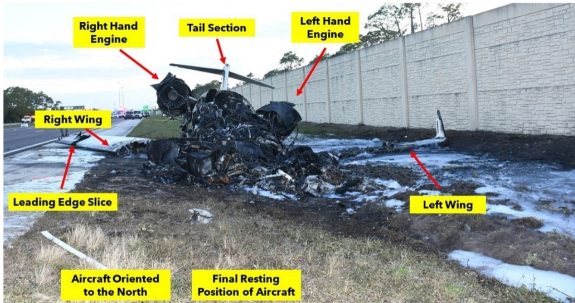
Figure 3. Main wreckage as found.
