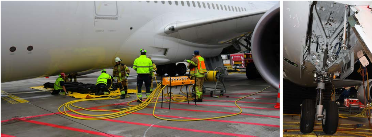
Fig. 6: Aircraft recovery (left) and extended nose landing gear (right)
