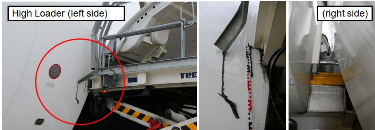
Fig. 4: Fuselage damage at the front cargo door
