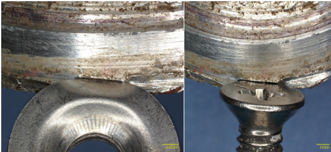
Figure 4. Impression marks on the counterweight plug consistent with contact with the washer (left) and screw (right).
