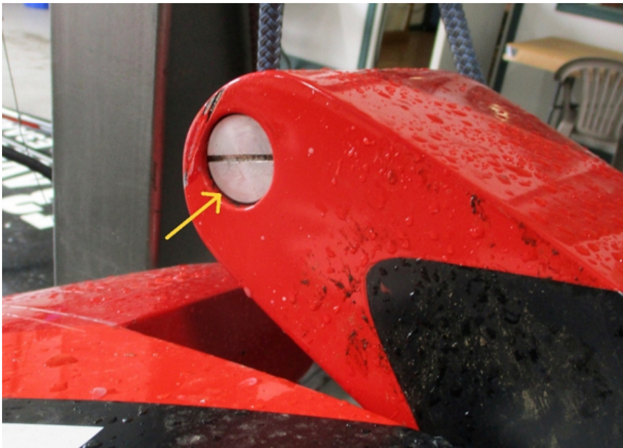
Figure 1. Counterweight plug as installed on the right elevator (postaccident photograph).
